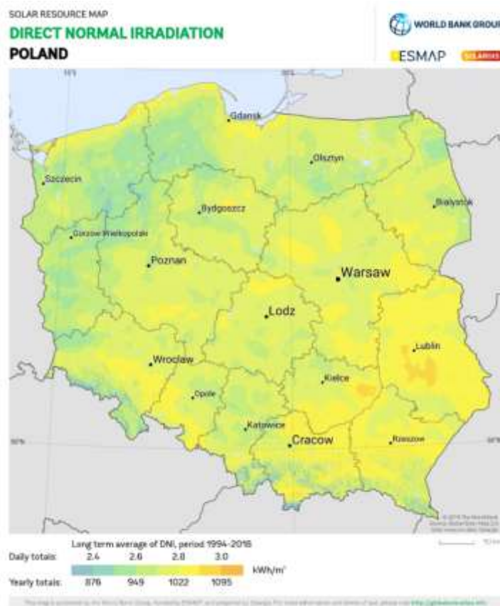
Figure 3 Long term average of direct solar irradiation (DNI) in Poland in kWh/m 2 .
